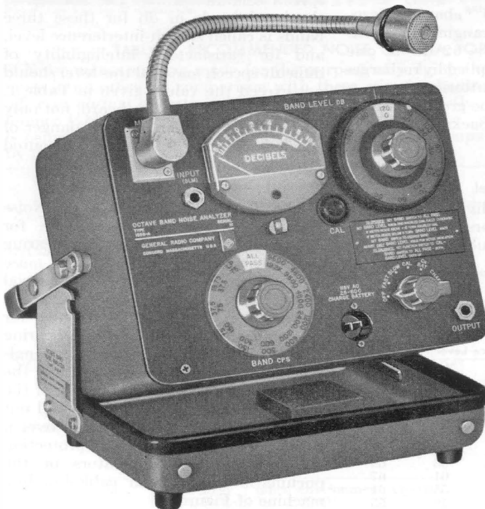
Figure 1. View of the Type 1558-A Octave-Band Noise Analyzer with the Type 1560-P4 PZT Microphone Assembly.
